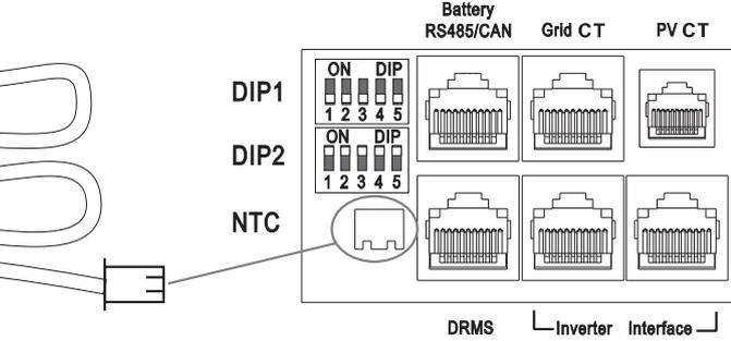
Connecting battery communication cable/NTC cable and clamps
