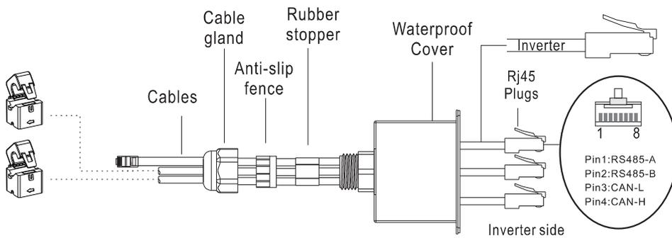
Step4: Insert the Rj45 plug of the network cable into the "RS485" place inverter until it snaps.
