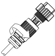
**f** Push threaded sleeve on to connection terminal until both are locked tightly
