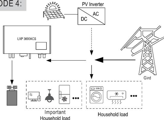
Battery can be charged by grid power (AC charge mode) by enable relevant functions and make right settings according to the real demands on the AC charge function via LCD operation, monitoring website or the APP.
