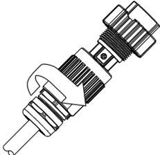
**f** Push threaded sleeve on to connection terminal until both are locked tightly
