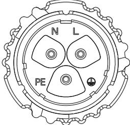
**d** Lead the UPS cable through cable gland, seal ring and threaded sleeve, and fully insert the conductors to corresponding terminals on connection terminal and tighten the screws.
