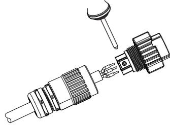
**e** Assemble the UPS connector and make sure that the rib of the terminal block and the groove on the housing engage perfectly.
