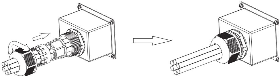
Step7: If lithium battery connecting the Battery communication cable the side with label of "Battery"(lithium battery ) to the lithium battery communication port .If lead-acid battery, just let the NTC near the lead-acid battery surface.
