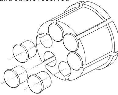
Step3: Put the Battery communication cable(lithium battery ) / "NTC" (lead-acid battery ) and CT cables cross into the cable gland, anti-slip fence, rubber stopper, waterproof cover one by one.
