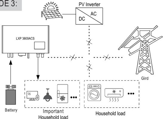
When grid power fails, immediately, the LXP 3600ACS discharges the battery power to the important household load using uninterrupted power supply technology which will guarantee the power supply stability and continuously of important loads. (Notice that it's required to enable the UPS function to activate this working mode)
