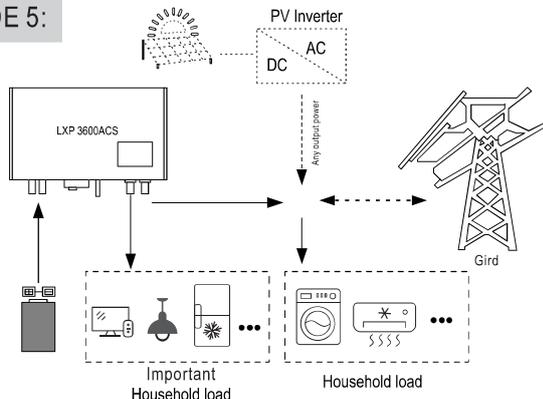
LXP 3600ACS can be set to "Force Discharge" mode, no matter PV inverter output energy is sufficient or not, the LXP 3600ACS discharges the power to the grid and Time & power & SOC limit can be set flexibly via LCD operation, monitoring website or APP.
